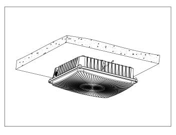
2. The fixed plate is fixed on the ceiling with a suitable screw.
