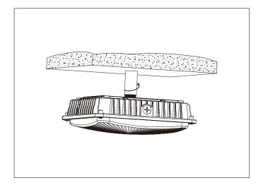
2. LED lamps with blades on the ceiling to the ceiling, the use of screws to be fixed. installation is complete
